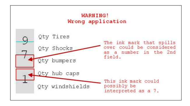
**How**: Make sure there's enough space between each field. You must re-design the document if that's the case. There's no minimum value that is required as the distance between 2 fields, except for the 7mm border that is required in order for the Anoto digital pen to recognize the pattern being used.
