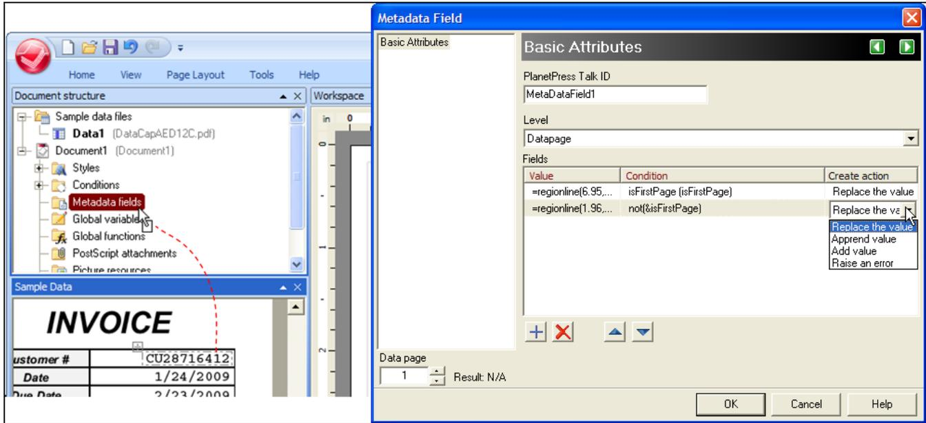
The Metadata Fields in the structure of a PlanetPress Design document allow to easily define documents or groups, by dragging and dropping data from the Sample Data directly onto the document's Metadata Fields.
