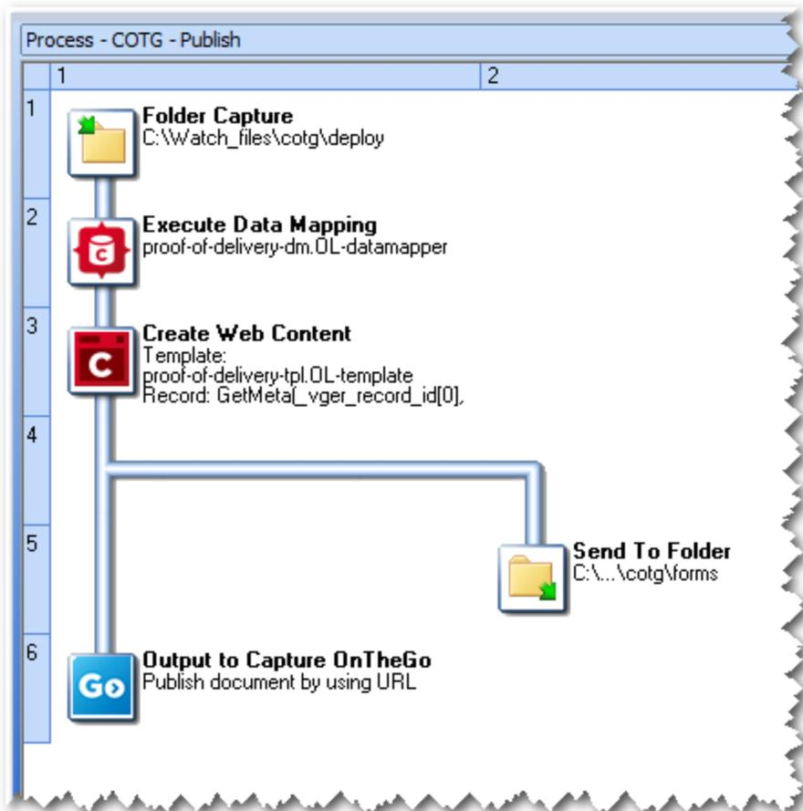
This process watches a certain folder. When a file enters that folder, a data mapping is performed on it. Then an HTML file is created and saved to another folder. The Output to PlanetPress Workflow plugin sends a ticket (not the actual HTML file) to the Capture OnTheGo Server, so that when the intended user logs in, the name of the HTML file will appear in the App's Repository, signaling to the user that the file is available for download.
