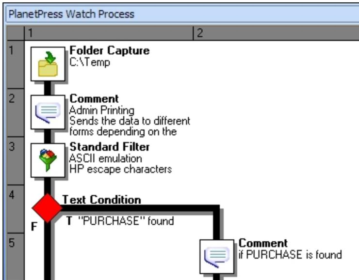
The numbers on the left indicate the task index, the folder capture being level 1 and the Text condition being on level 4.
