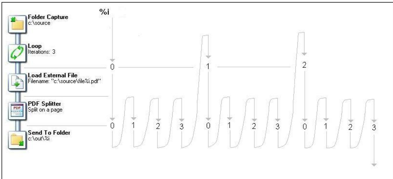
**Initial input tasks do not modify the value of  $\%i$ . However, the following tasks do trigger the variable:**
