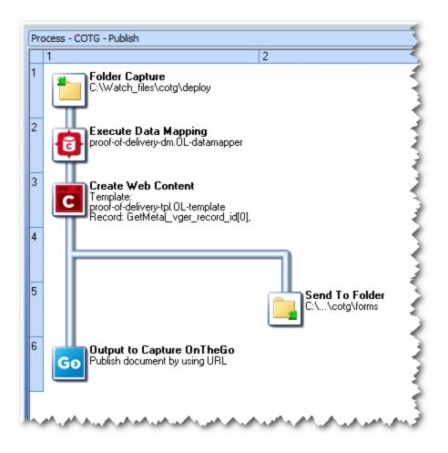
This process watches a certain folder. When a file enters that folder, a data mapping is performed on it. Then an HTML file is created and saved to another folder. The Output to Capture OnTheGo plugin sends a ticket (not the actual HTML file) to the Capture OnTheGo Server, so that when the intended user logs in, the name of the HTML file will appear in the App's Repository, signaling to the user that the file is available for download.
