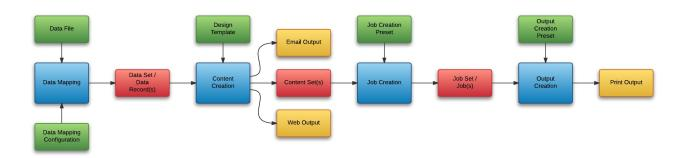
Typically an individual workflow process (shown above in *blue*) will take one or more input files as input (shown above in *green*), and will produce either intermediary output in the form of a data entity (shown above in *red*), or final output in the form of print, web, or email based content (depending on the context of the content produced) (shown above in *yellow*).
