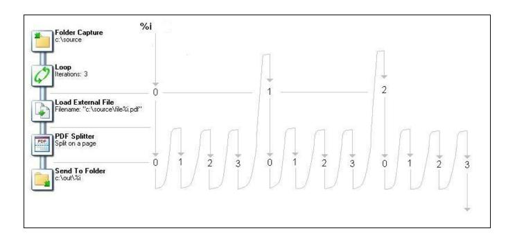
Initial input tasks do not modify the value of %i. However, the following tasks do trigger the variable:
