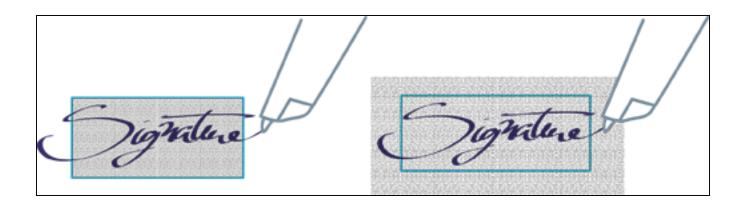
This is because the pen's camera (which captures the position of the pen) is located under the pen tip and must fully see the pattern. The following image illustrates how the pen reads its position:
