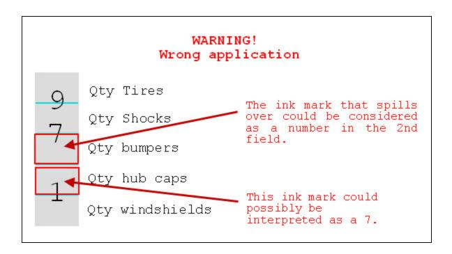
**How**: Make sure there's enough space between each field. You must re-design the document if that's the case. There's no minimum value that is required as the distance between 2 fields, except for the 7mm border that is required in order for the Anoto digital pen to recognize the pattern being used.
