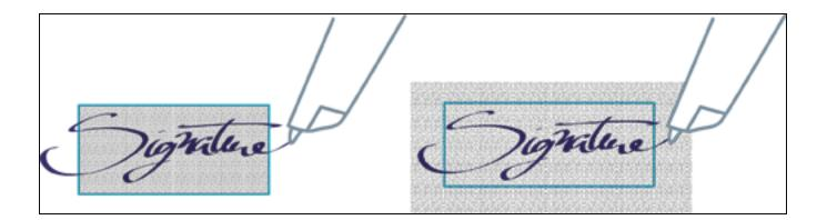
This is because the pen's camera (which captures the position of the pen) is located under the pen tip and must fully see the pattern. The following image illustrates how the pen reads its position:
